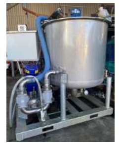
Mixing tank with recir.culated GJ
